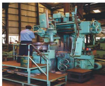
Piston crown for diesel engines are ground to an accuracy of 0.01 mm on our Vertical Turret Lathes. This tolerance is lowered to a much higher accuracy whenever required. Also machine is equipped with DRO (Digital Read Out) for accurate machining.
