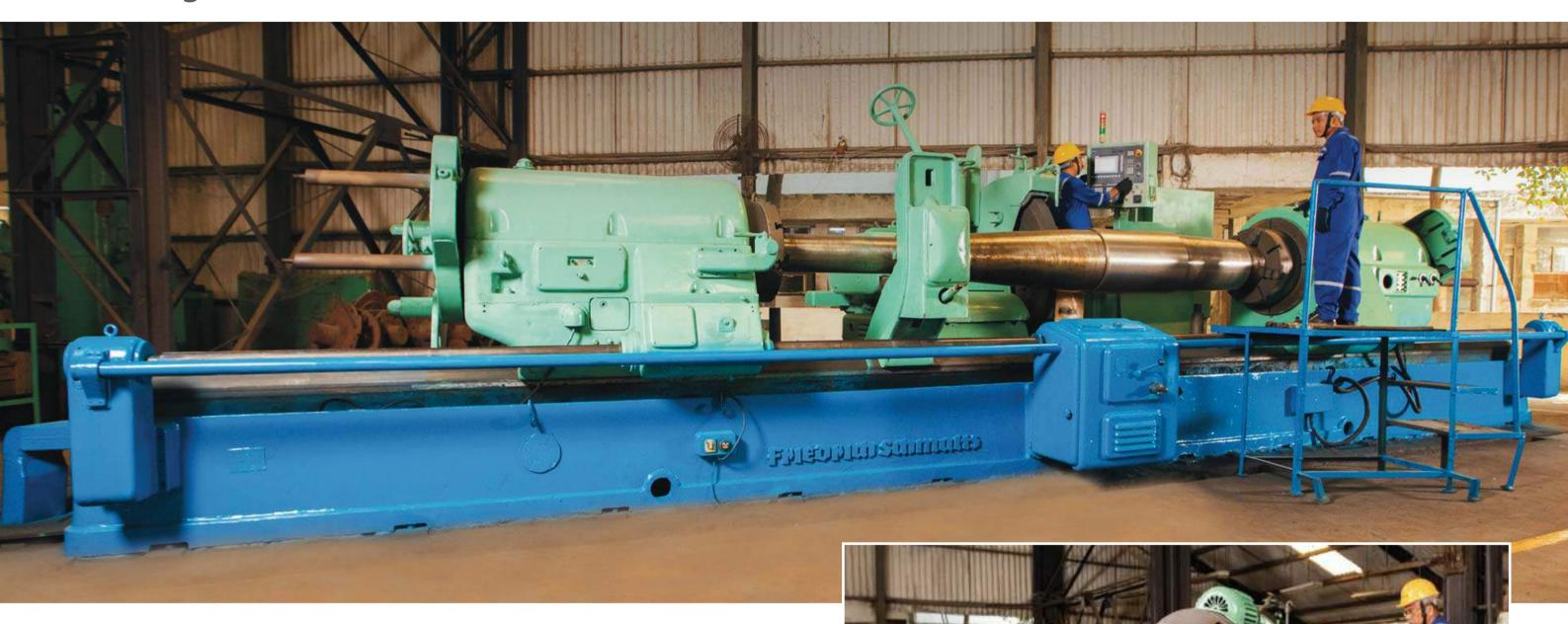
Friedrich Schmalts make German Cylindrical cum Crank shaft grinding machine equipped with CNC controller. At United Van Der Horst we ensure that jobs are immediately undertaken for precision grinding. We are capable to grind various jobs with an accuracy of 0.01 mm i.e. 10 microns and surface finish of Ra value less than 0.4 micron.
